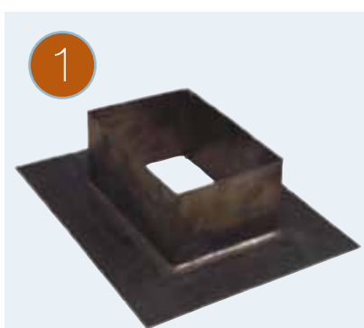
1 Pre-formed, shaped lead slate made with allowance for thermal movement, a minimum of a 75mm upstand and 50mm flange for lap welding to the roofing bays.
